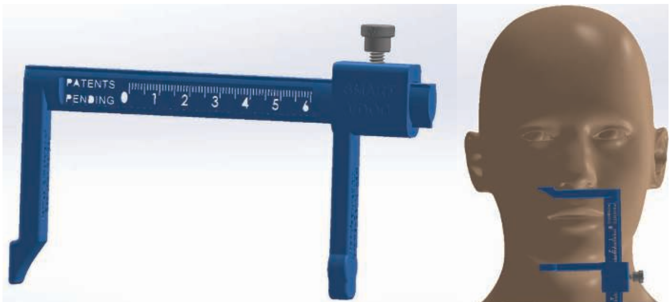
Using a caliper, closed OVD can be rapidly determined and recorded using fixed anatomic landmarks.
