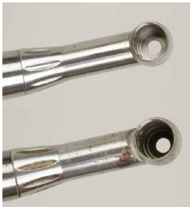
Figure 7: A body or shell before (top) and after (bottom) the corrosive effects of sterilization over time
