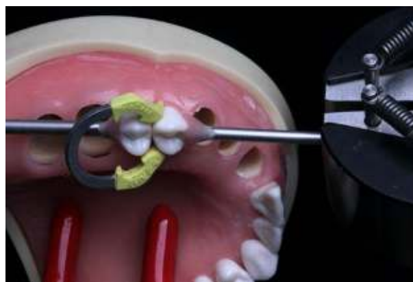
FIGURE 6: Two typodont premolar teeth with a metal rod placed into the mesial surface of the first premolar and the distal surface of the second premolar.
