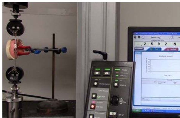
FIGURE 5: Custom testing fixture for measuring separating force.
