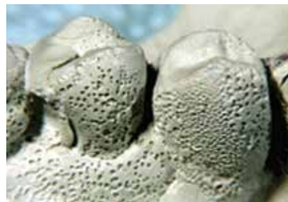
FIGURE 21: The cast is covered with multiple bubbles resulting from hydrogen gas release from the VPS material due to pouring of cast too early.
