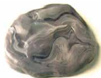
FIGURE 19: Streaking of the impression material resulting from inadequate mixing.
