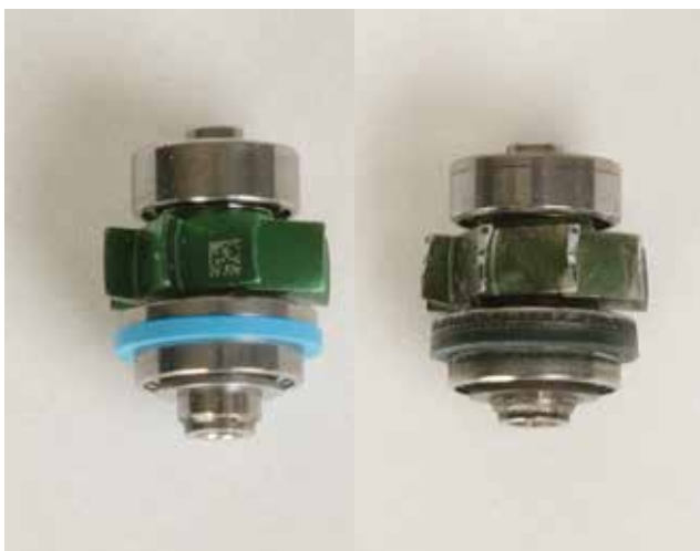
Figure 8: High-speed turbine before (left) and after (right) the effects of wear and sterilization
