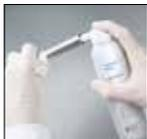
Place appropriate nozzle on Midwest® Plus Aerosol Spray (380080M). While holding can upright, insert nozzle fully into the handpiece/attachment/motor. For fixed backend handpieces or motors, place the tip of the nozzle into drive air tube.
