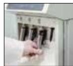
Position handpiece/attachment/motor onto the appropriate maintenance adapter.
