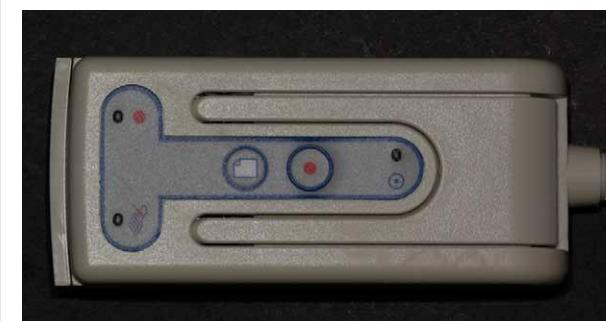
Figure 2. 85u thick plastic disposable sensor. The lines contain ink that changes resistance with pressure, generating force data.
