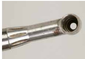
Figure 9. Corrosive effects of sterilization
