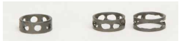
Figure 14. Bearing retainer showing stages of degradation
