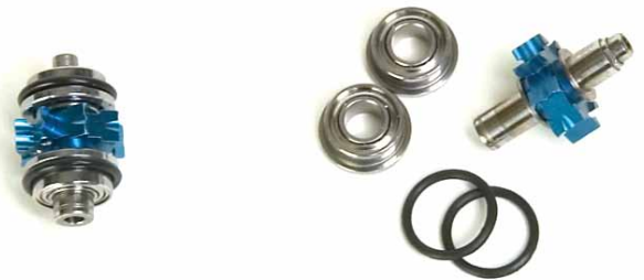
Figure 19. Turbine assembled and unassembled
