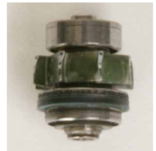
Figure 10. High-speed turbine Figure 11. Effects of wear and sterilization
